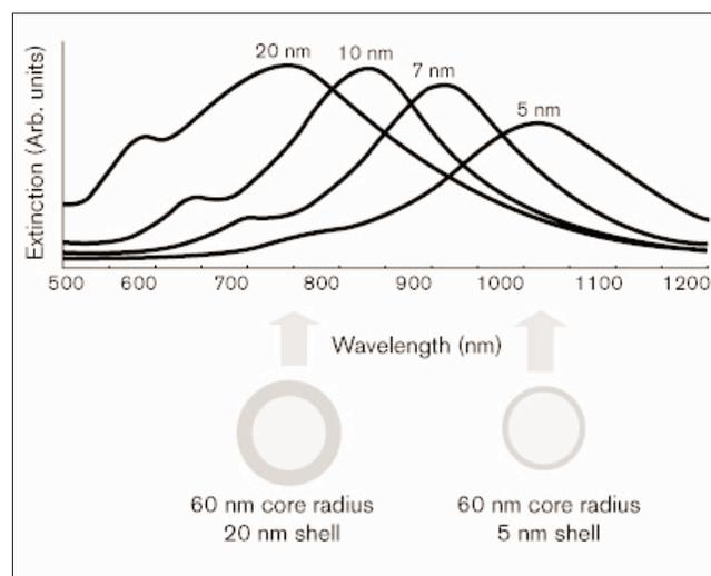
Optical resonances of gold-shell–silica-core nanoshells, as a function of their core : shell ratio, for particles of 120 nm core diameter. Respective spectra correspond to the nanoparticles depicted beneath. Reproduced from [8] with permission.
