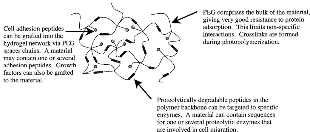
**Figure 3.** Schematic diagram depicting the structure of the hydrogel materials used in these studies as ECM analogs
