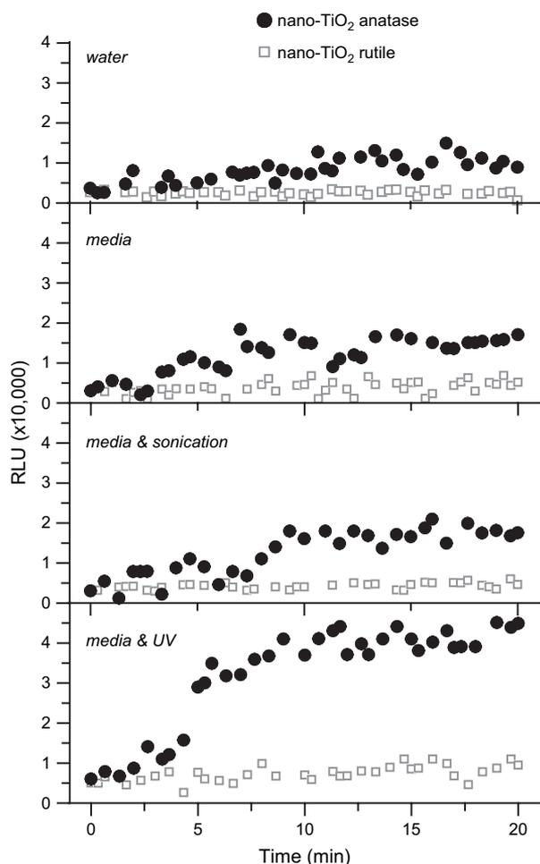
**FIG. 7.** *Ex vivo* determination of reactive oxygen species in nano-TiO<sub>2</sub> suspensions. The panel shows the emission of light from luminol ( $\lambda = 416$  nm) in the presence of nano-TiO<sub>2</sub> anatase particles and nano-TiO<sub>2</sub> rutile particles in (A) water, (B) Dulbecco's Modification of Eagle's Media, (C) media and sonication, and (D) media and UV light. The concentrations of the nano-TiO<sub>2</sub> samples are both 15 mg/ml.
