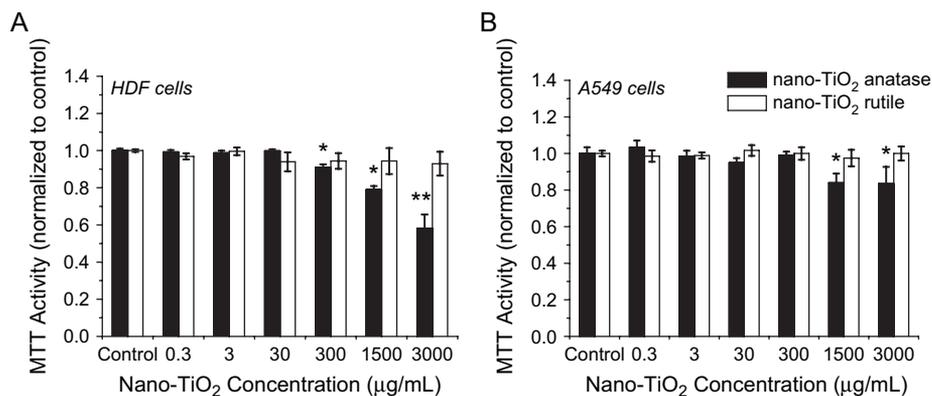
**FIG. 5.** The mitochondrial activity (MTT activity) of (A) HDF and (B) A549 cells after 48 h exposure to nanoscale TiO<sub>2</sub> anatase and rutile phases. Results are combined from three independent exposures. Groups significantly different from the control group (by ANOVA  $p_{\text{HDF}} < 0.00231$  and  $p_{\text{A549}} < 0.00197$  followed by Dunnett's test) are shown by \* $p < 0.05$  or \*\* $p < 0.01$ .
