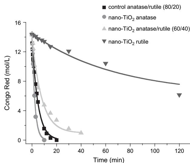
**FIG. 8.** Photodegradation of aqueous Congo red (10 mg/l, 14  $\mu$ mol/l) in the presence of various nano-TiO<sub>2</sub> catalysts (1 g/l). Based on this plot, the per gram efficiencies of the TiO<sub>2</sub> powders increased in the order nano-TiO<sub>2</sub> rutile particles < nano-TiO<sub>2</sub> anatase/rutile particles < control anatase/rutile < nano-TiO<sub>2</sub> anatase particles.
