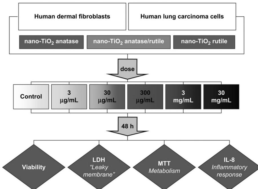
**FIG. 2.** Flowchart of experimental protocol for testing the cellular response with HDF and A549 cell lines to nano-TiO<sub>2</sub>. Cultured cells were dosed with nano-TiO<sub>2</sub> anatase and rutile particles for all experiments and nano-TiO<sub>2</sub> anatase/rutile particles for cell viability experiments. Cells were exposed to nano-TiO<sub>2</sub> particles at various concentrations (3 µg/ml–3 mg/ml), incubated for 48 h, and tested for different biochemical endpoints.
