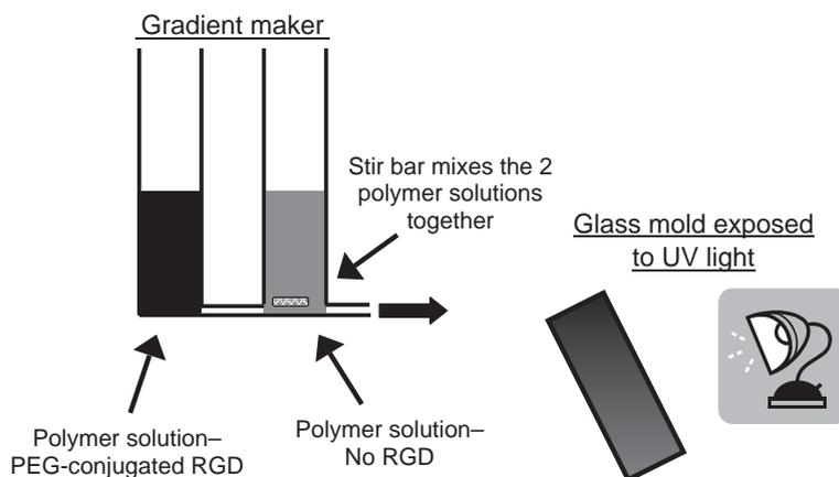
Fig. 1. Gradient hydrogels were formed using a gradient maker as depicted above in combination with a peristaltic pump to control the combination of polymer solutions with and without BSA. The resulting polymer solution is then pumped into a mold where it is exposed to UV light to stabilize the concentration gradient.
