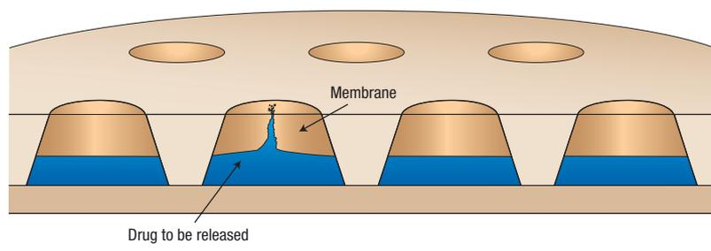
**Figure 2** The polymer-based microchip drug-delivery devices designed to release many doses of drug over time<sup>1</sup>. The base of the microchip was made of a slowly degrading polymer, poly(L-lactic acid). Reservoirs were formed in the base, filled with drug solutions, and then sealed with polymer membranes. The composition of each membrane can be varied so that doses of drug are released at the desired times.
