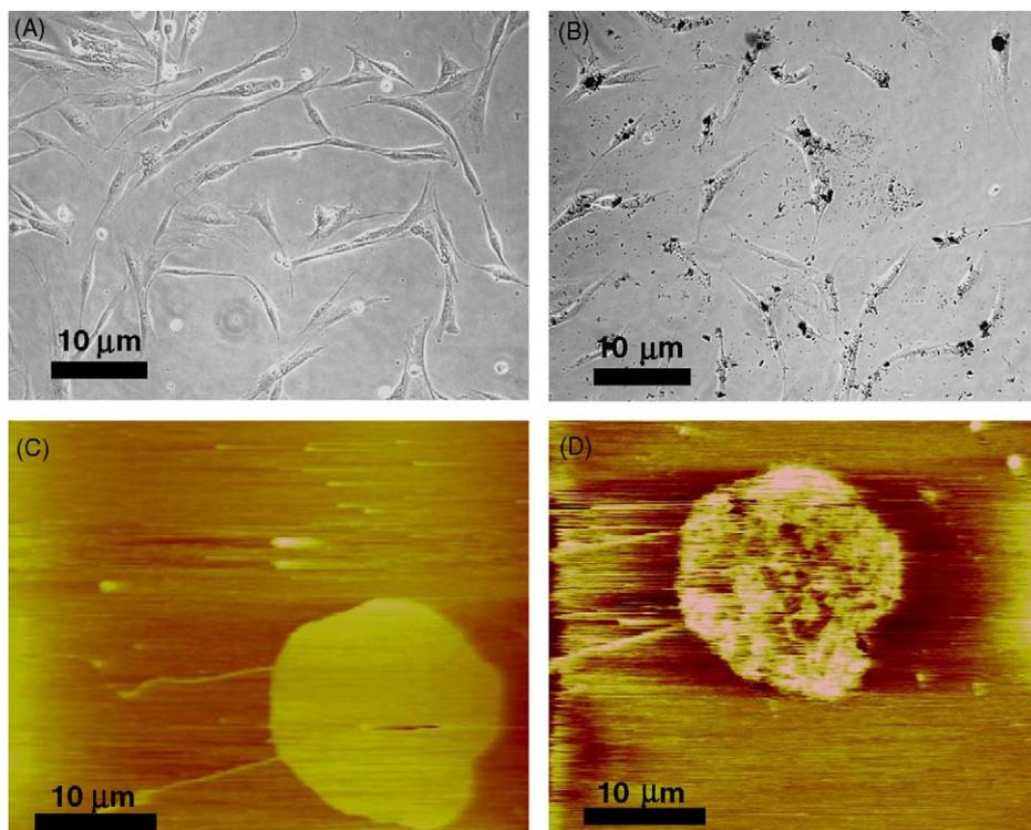
Fig. 4. SWNT-phenyl-SO<sub>3</sub>H preferentially deposit on the DOPC membrane. Optical micrographs of (A) healthy HDFs before exposure and (B) HDFs after exposed to SWNT-phenyl-SO<sub>3</sub>H for 48 h. Atomic force micrographs of (C) intact DOPC membrane and (D) DOPC membranes exposed to SWNT-phenyl-SO<sub>3</sub>H for 2 h.
