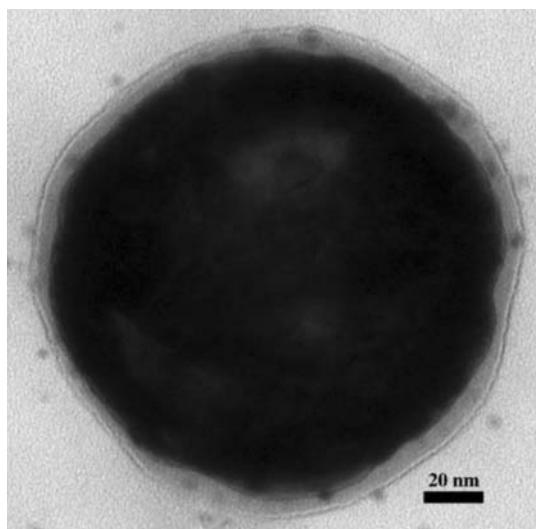
**Fig. 3** A transmission electron microscope image of a gold-silica nanoshell that has been PEGylated and conjugated to anti-HER2 antibodies. The antibodies have been tagged with gold beads for visualization.
