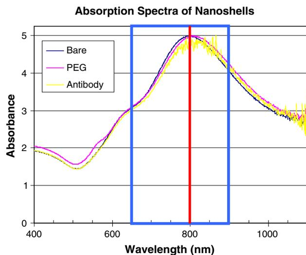
**Fig. 2** The absorption spectra for bare nanoshells, PEGylated nanoshells, and antibody conjugated nanoshells was obtained using a spectrophotometer. The data is normalized to a peak absorbance of 5, to which all nanoshells were diluted prior to use. The red line at 800 nm indicates the wavelength of the laser that was used for our treatments. The blue box indicates the near infrared window
