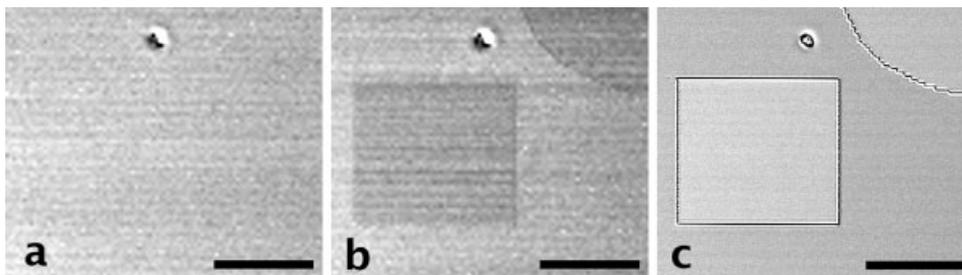
**Figure 8.** Another advantage of LSL is the ability to observe exposed regions of photoresist with DIC imaging before developing. **a**: Unexposed photoresist was imaged with a non-destructive 514 nm argon laser to locate the surface. **b**: Following LSL with a 458 nm argon laser, the 514 nm laser was again used to image the exposed regions. **c**: Confirmation that the regions of increased contrast were exposed during LSL is seen in the developed photoresist. Scale bar = 50  $\mu\text{m}$ .
