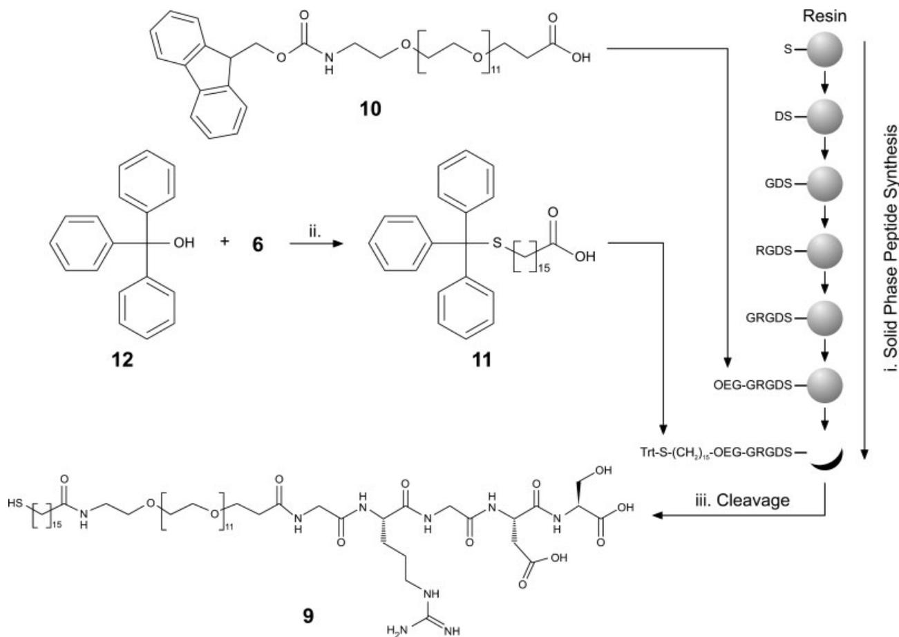
**Figure 3.** Synthesis of thioalkane-OEG-GRGDS by solid-phase peptide synthesis (SPPS). (i) Solid-phase peptide synthesis (SPPS) via the Fmoc strategy, (ii) neat TFA; evaporation; diethyl ether extraction, (iii) 95% TFA, 2.5% H<sub>2</sub>O, 2.5% TIPS.
