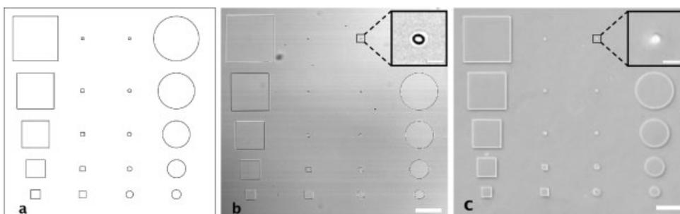
**Figure 9.** Replica-molding of poly(dimethylsiloxane) (PDMS) from a photoresist master created with LSL. **a**: Virtual mask drawn onscreen, **(b)** developed photoresist master, and **(c)** replica molded PDMS. Scale bar = 100  $\mu\text{m}$ . The minimum feature size achieved with a  $10\times$  objective (NA 0.45) was 3  $\mu\text{m}$  (enlarged in **b**, **c**; scale bar = 5  $\mu\text{m}$ ).
