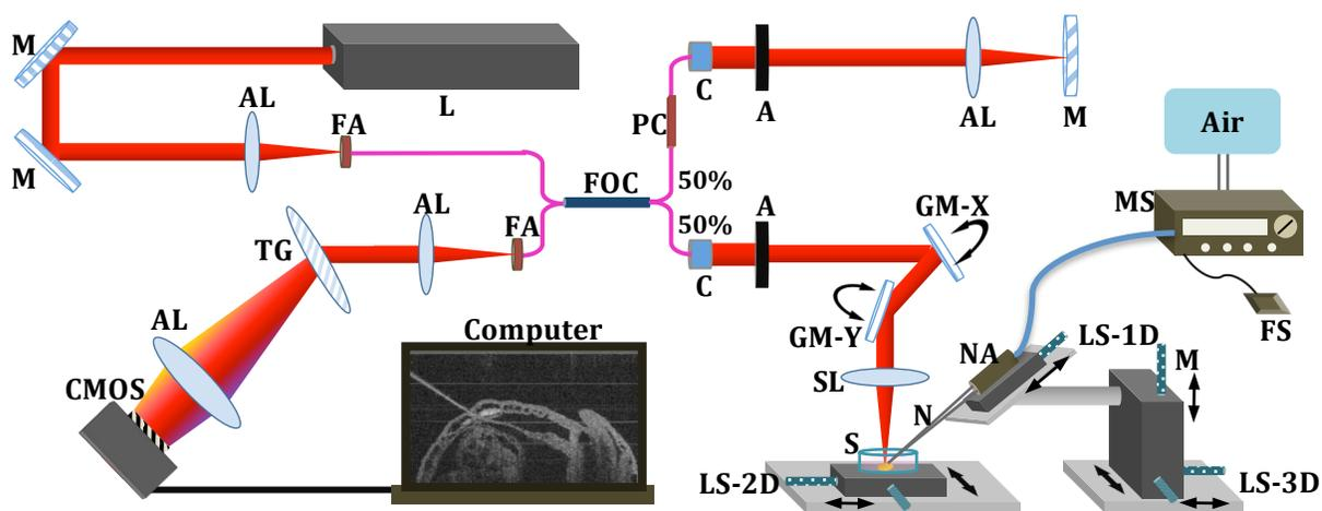
**Figure 1. Experimental setup for OCT guided injections.** L – laser, M – mirror, AL – achromatic lens, FA – fiber adaptor, TG – transmission grating, FOC – fiber optics coupler, PC – polarization controller, C – collimator, A – aperture, GM-X – galvo mirror-X, GM-Y – galvo mirror-Y, SL – scan lens, S – sample, N – needle, NA – needle adaptor, M – Micrometer, LS-1D – 1-D linear stage, LS-2D – 2-D linear stage, LS-3D – 3-D linear stage, MS – microinjection system, FS – foot switch.
