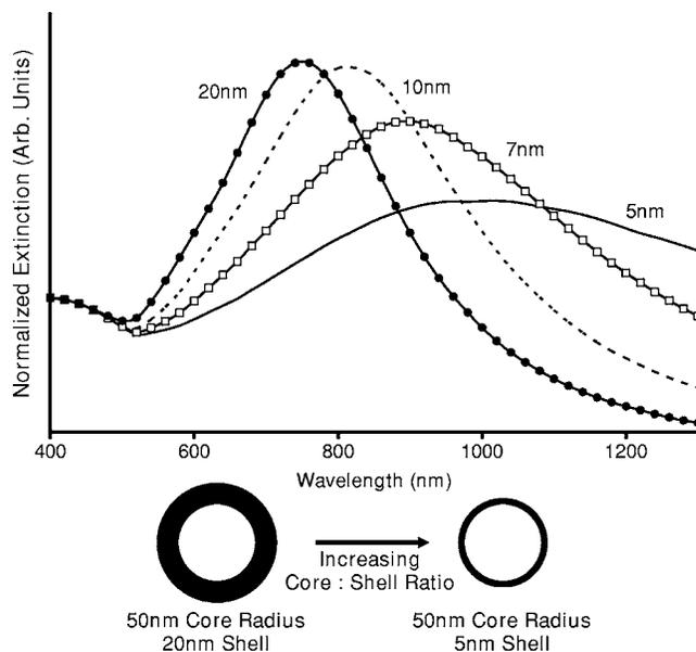
**Fig. 1** By increasing the core radius to shell thickness ratio, the peak extinction resonance can be shifted well into the NIR. For gold nanoshells with a core (silica) radius of 50 nm and a decreasing gold shell thickness, the peak resonance shifts to longer wavelengths.
