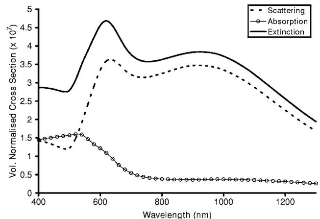
**Fig. 5** Volume normalized cross sections of the R75/115 gold nanoshell ( $n=1.4$ ). Although the scattering property of the nanoshell generally dominates the absorption, it is expected that the diffuse reflectance of tissue with nanoshells will decrease across wavelength.
