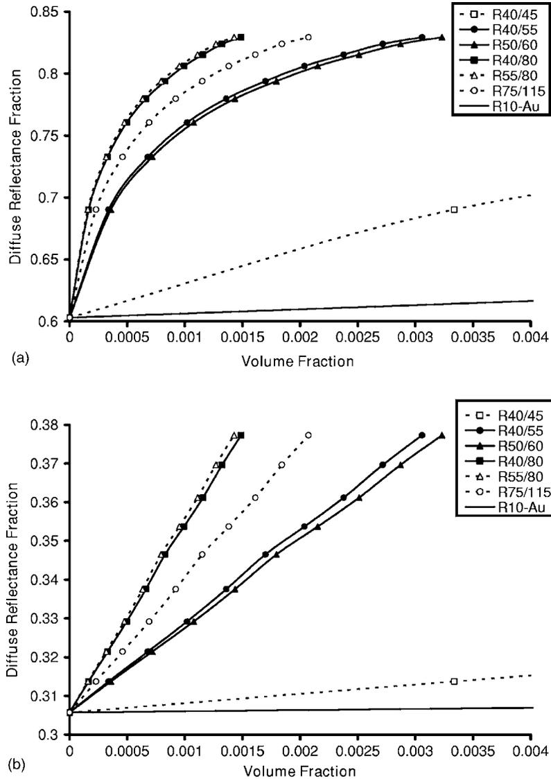
**Fig. 6** Diffuse reflectance from the (a) bulk (model A-1) and (b) multilayered (model B-1) models with  $\mu_{abs(c)}=0.05 \text{ cm}^{-1}$ , using different types of nanoparticles. The higher the volume-normalized scattering cross section, the more the diffuse reflectance increases with the same volume fraction of nanoshells added. The results show the studies that neglected absorption from the nanoparticles, assuming the particles as simple scatterers.
