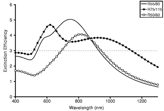
**Fig. 4** Representative extinction efficiencies of three different nanoshells, R75/115, R50/60, and R55/80, used in the Monte Carlo experiments. The different extinction profiles are plotted against a broad wavelength range, showing optical activity well into the NIR. Nanoshells of different sizes produce unique and different optical responses.
