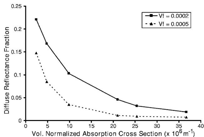
**Fig. 8** The diffuse reflectance as a function of the volume normalized absorption cross section of different gold nanoshells used in the multilayered Monte Carlo studies (refer to Table 1). As the volume normalized absorption increases, the reflectance correspondingly decreases. Volume fractions ( $V_f$ ) of 0.0002 and 0.0005 are shown, within the constraints for independent scattering.
