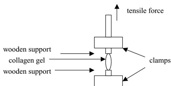
**FIGURE 1.** Collagen gels were attached to balsa wood using a cyanoacrylate glue to mediate the clamping of gels. Tensile testing was performed using Vitrodyne V1000 with a strain rate of 100  $\mu\text{m}/\text{sec}$  using a 150 g loading cell.
