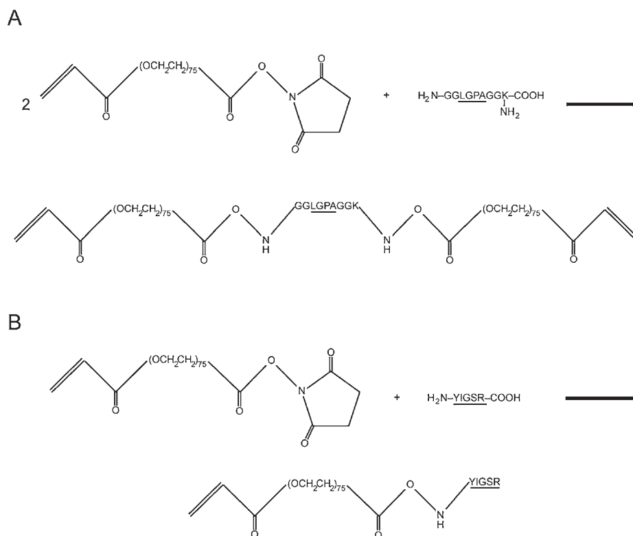
FIG. 1. (A) Coupling of collagenase-sensitive peptide, LGPA, with acryl-PEG-NHS to form a degradable hydrogel, ABA block copolymer, terminated in acrylate groups for photopolymerization. (B) Coupling of cell-adhesive peptide, YIGSR, with acryl-PEG-NHS to facilitate preadipocyte binding to hydrogel. 21
