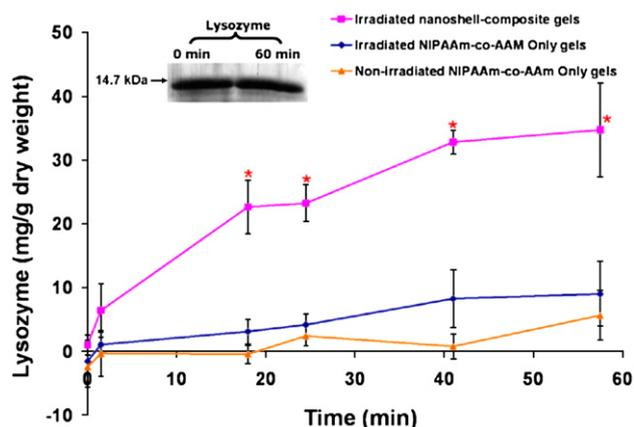
Fig. 8. Release of lysozyme (mg/g dry weight represents mg of lysozyme released/g of polymer dry weight) from irradiated nanoshell-composite hydrogels (square), irradiated NIPAAm-co-AAm hydrogels (diamond), and nonirradiated NIPAAm-co-AAm hydrogels (triangle) as a function of time. SDS-PAGE gel for lysozyme control taken from protein solution used to swell hydrogels (0 min) and for lysozyme released after 60 min laser irradiation (60 min). Data reported as mean  $\pm$  SD,  $n = 3$ .
