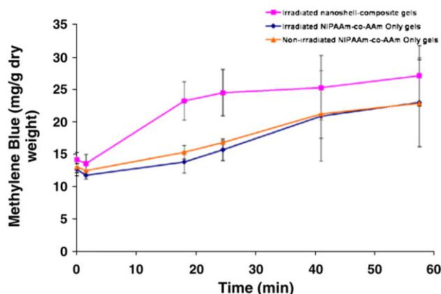
Fig. 6. Release of methylene blue (mg/g dry weight represents mg of methylene blue released/g of polymer dry weight) from irradiated nanoshell-composite hydrogels (square), irradiated NIPAAm-co-AAm hydrogels (diamond), and nonirradiated NIPAAm-co-AAm hydrogels (triangle) as a function of time. Data reported as mean  $\pm$  SD,  $n = 3$ .
