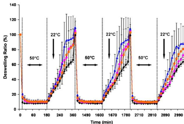
Fig. 3. Reversible thermal behavior of NIPAAm-co-AAm control hydrogels (diamond) and nanoshell-composite hydrogels with varying concentrations of SiO<sub>2</sub>-Au nanoshells (circle=2×10<sup>9</sup> nanoshells/mL; triangle=4×10<sup>9</sup> nanoshells/mL; square=6×10<sup>9</sup> nanoshells/mL) showing reversible collapse of the hydrogels at 50 °C followed by hydrogel reswelling at 20 °C as a function of time. Data reported as mean±SD, n=3.
