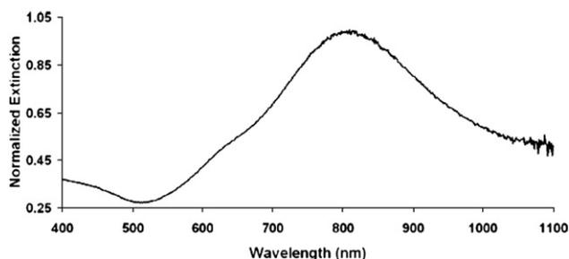
Fig. 1. The normalized extinction spectrum of fabricated  $\text{SiO}_2\text{-Au}$  nanoshells with peak at 804 nm.
