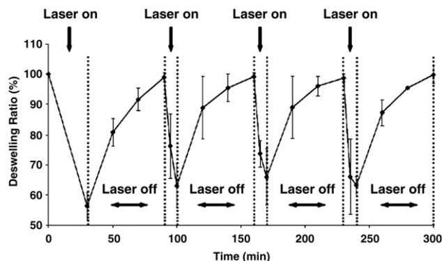
Fig. 5. Reversible photothermal behavior of composite hydrogels with 2×10<sup>9</sup> nanoshells/mL showing collapse and reswelling of the hydrogels during and after laser irradiation as a function of time. Data reported as mean±SD, n=3.
