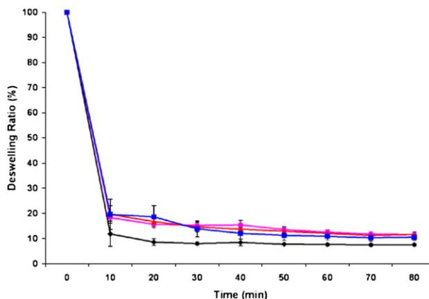
Fig. 2. Thermal deswelling of NIPAAm-co-AAm control hydrogels (diamond) and nanoshell-composite hydrogels with varying concentrations of  $\text{SiO}_2\text{-Au}$  nanoshells (circle= $2 \times 10^9$  nanoshells/mL; triangle= $4 \times 10^9$  nanoshells/mL; square= $6 \times 10^9$  nanoshells/mL) at  $50 \text{ }^\circ\text{C}$  as a function of time. Data reported as mean  $\pm$  SD,  $n=3$ .
