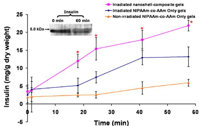
Fig. 7. Release of insulin (mg/g dry weight represents mg of insulin released/g of polymer dry weight) from irradiated nanoshell-composite hydrogels (square), irradiated NIPAAm-co-AAm hydrogels (diamond), and nonirradiated NIPAAm-co-AAm hydrogels (triangle) as a function of time. SDS-PAGE gel for insulin control taken from protein solution used to swell hydrogels (0 min) and for insulin released after 60 min laser irradiation (60 min). Data reported as mean  $\pm$  SD,  $n = 3$ .
