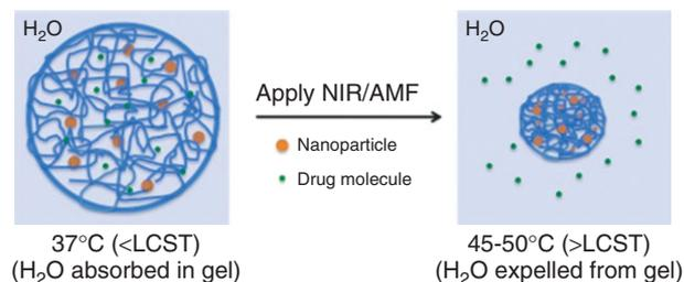
**FIGURE 3** | Schematic of drug delivery from bulk hydrogels.
