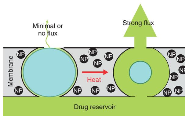
**FIGURE 5** | Schematic of drug delivery from magnetically triggered nanogel composite membrane. (Reprinted with permission from Ref 52. Copyright 2009 American Chemical Society)
